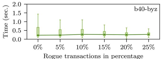
Fig. 17: Latency vs. ratio of rogue transactions.
