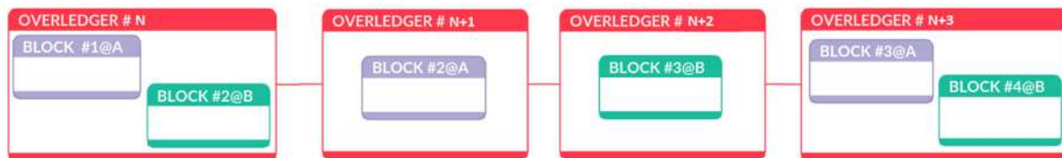
Fig. 17: Overledger modelled as a blockchain of block set 4.6. Note that the block 2 and 3 can be grouped together.
